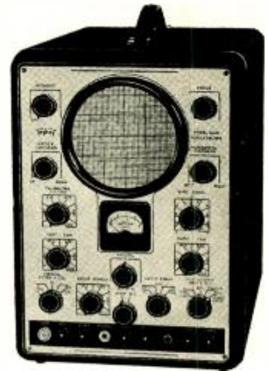
A commercial oscilloscope with built-in 10-range voltage source and meter for peak-to-peak screen-scale calibration.
